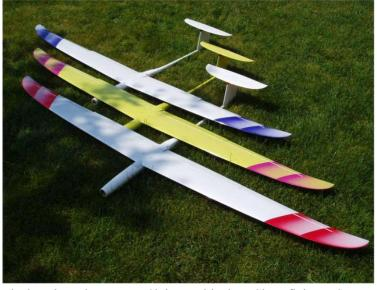
materials and design are especially for constest flying. Never the less the Raketenwurm 2b is a multi talent. Slope flying, DS flying is also possible with the Raketenwurm 2b. The surface has only a minimum amount of colour. It saves a lot weight and gives the model a special character. The wing is produced out of full carbon and the fuse out of aramid with unidirectional carbon. The Raketenwurm 2b is nearly ready to fly. Never the less we recommend to read the instruction very carefully.
