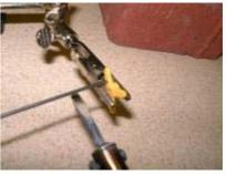
Bend a "z" at the end of the pushrod. Glue the servohorns into the aileron and flap. Be careful that the horns have absolute
