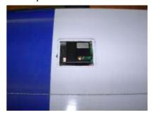
Make wiring of the servocables and lead them to the back-middle of the wing.
